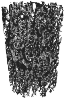
micro-CT @ 22 \mu\text{m} resolution \phi : 8 mm H: 15 mm
