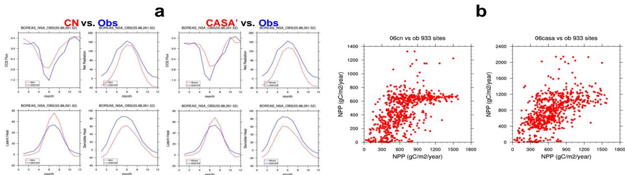
**Figure 2.** Example model-to-observation comparison diagnostics for (a) surface CO<sub>2</sub> and energy balance at the BOREAS Fluxnet site and (b) NPP at Ecosystem Model-Data Intercomparison (EMDI) sites from CLM3-CN and CLM3-CASA' for the control run (Experiment 1.1).
