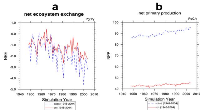
**Figure 3.** Example model-to-model comparison diagnostics for (a) NEE and (b) NPP for CLM3-CN and CLM3-CASA' from the varying climate, CO<sub>2</sub>, and N deposition run (Experiment 1.4).
