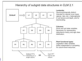
Columns: Store and all state variables. Geospatially discrete. Resolved over one or more (plant, soil, etc.) heterogeneity or sub-resolution scales.
