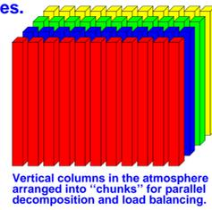
Vertical columns in the atmosphere arranged into "chunks" for parallel decomposition and load balancing.
